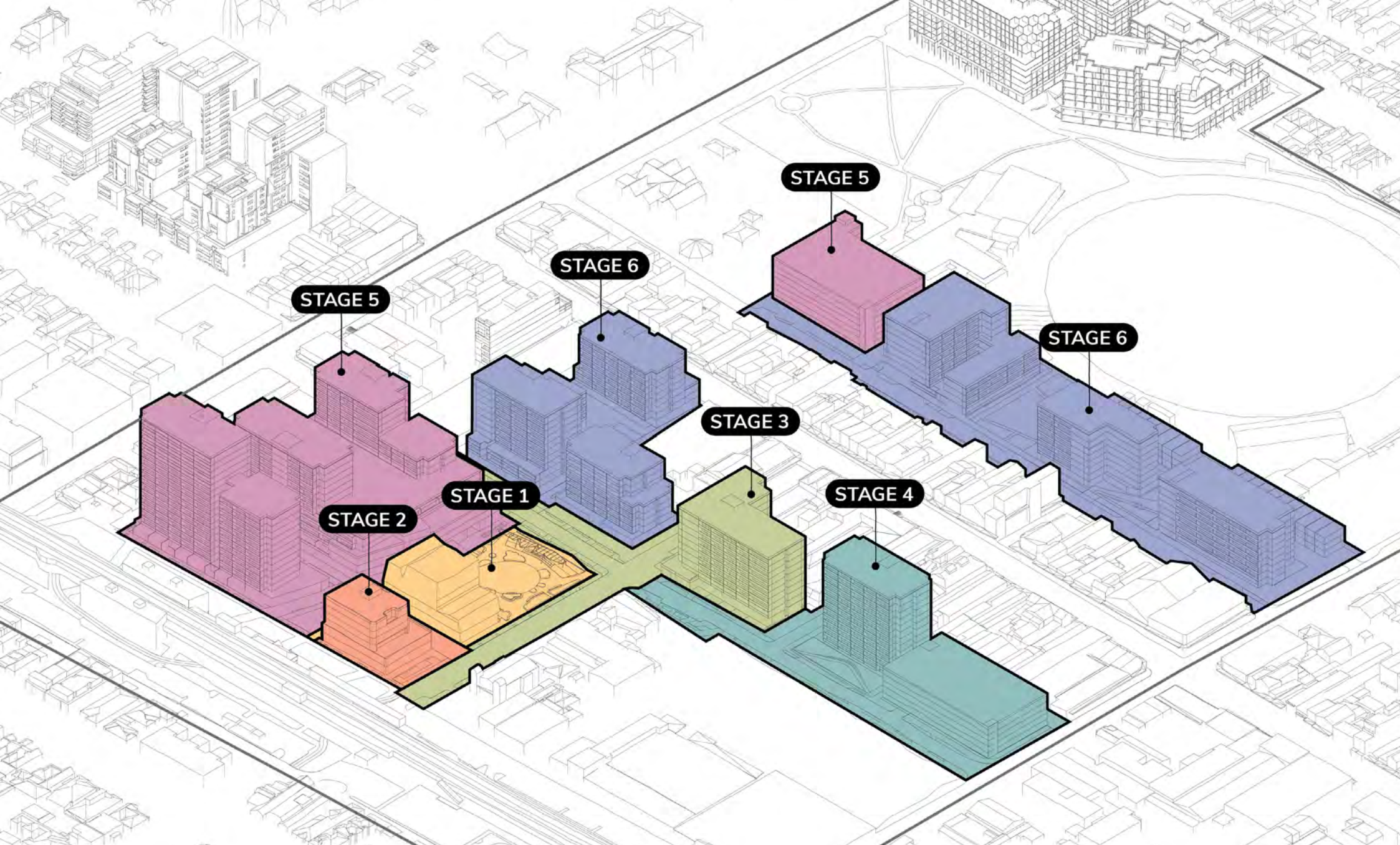
Potential staging. Indicative image by MGS Architects.
